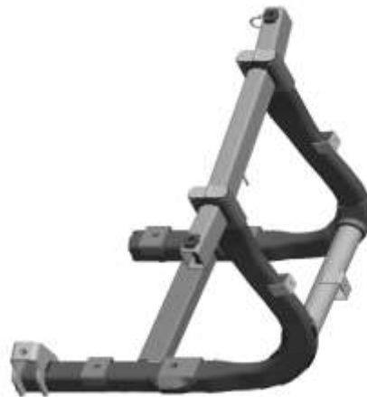
Fig.7: Modified design of engine supporting bracket for 3-D Model
